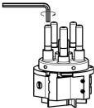
Fig.69: Loosening the contact pin
